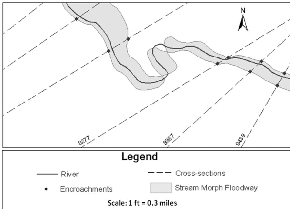
**Figure 7: Helical patterns in the stream morph method. Such patterns cannot be avoided at the meanders where there are no cross-sections**
