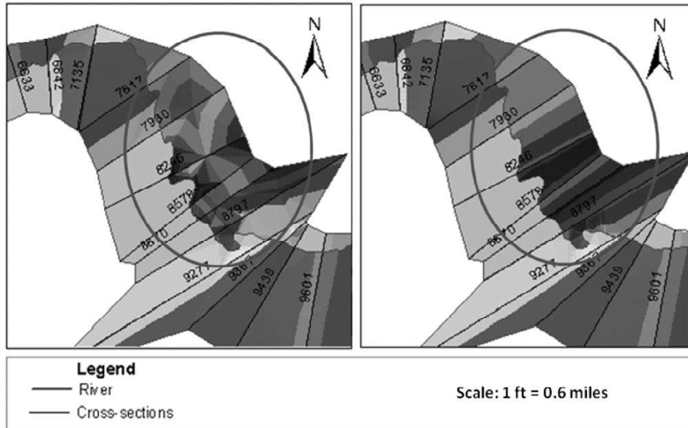
**Figure 11: Improvements in TIN triangulation due to densification. Improper triangulation due to lack of definition (left) and improved triangulation after densification (right)**
