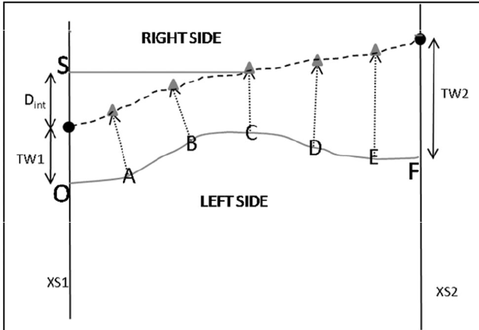
Figure 3: Schematic of the normal distances method. The method is based on plotting floodway boundary by intersecting the normal lines at each vertex to the interpolated width line
