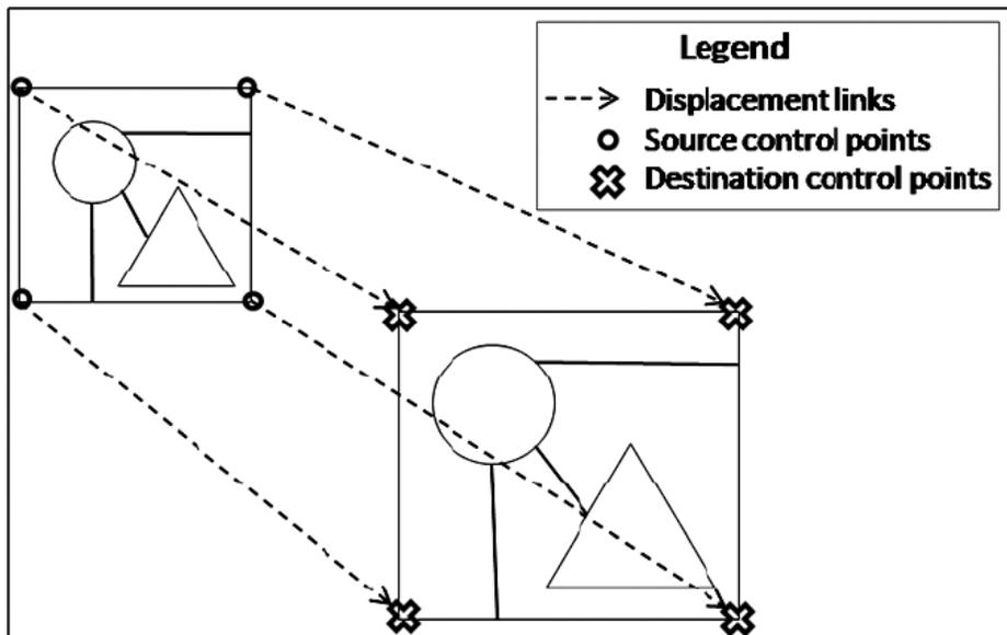
Figure 1: Principle behind transformation techniques (adapted from ArcGIS help documentation)
