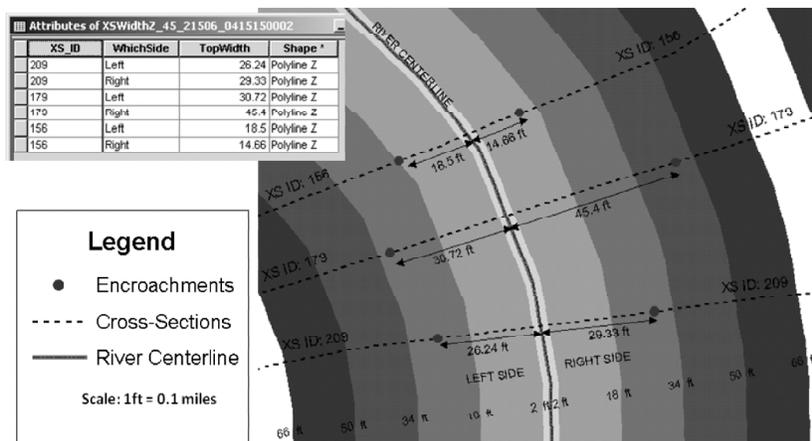
**Figure 4: Concentric buffer rings between cross-sections 156 and 209. The width of each concentric ring is shown at the bottom. The width is same on the left and right side of the river centerline. These rings are converted into a TIN to create the BufferTIN.**
