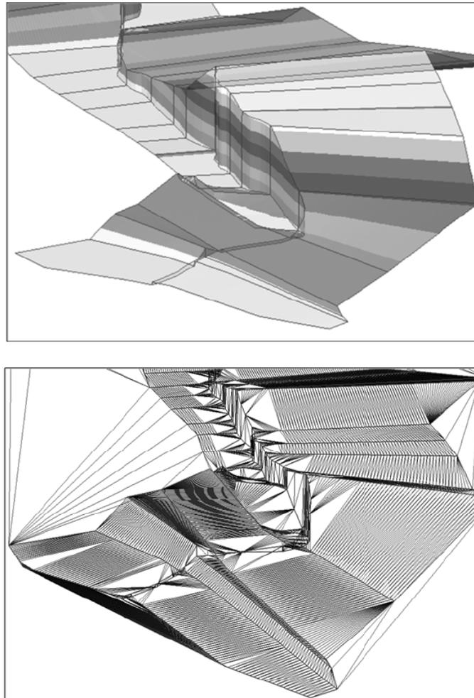
**Figure 12:**Elevation ‘wall’ along the river centerline. The widths of the floodway are larger on the right side than the left side. Hence, the XSTIN indicates lower values on the left side compared to the right side of the river (Top). The TIN triangulations show the vertical TIN faces along the river centerline which prevents triangulations from one side of the river from affecting the other side (Bottom)
