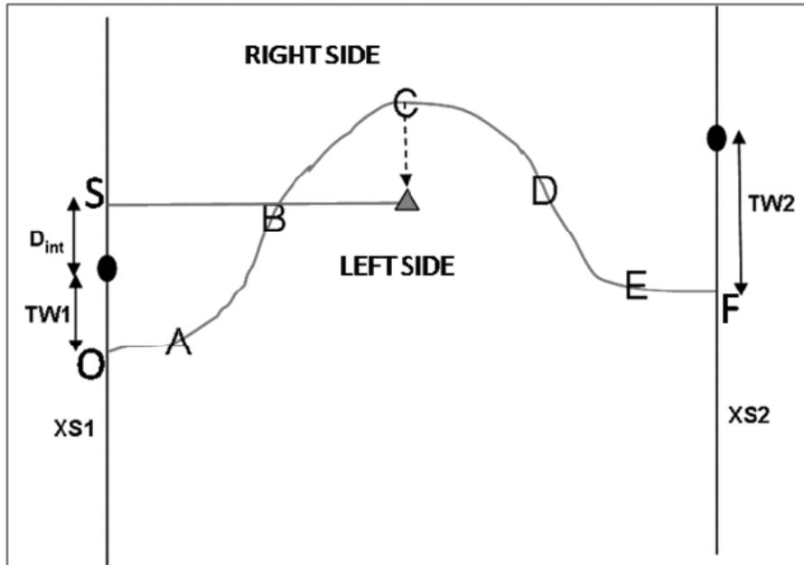
Figure 8: Problem with the normal distances approach. At narrow topwidth cross-sections, the intersection point will be identified on the wrong side of the river centerline
