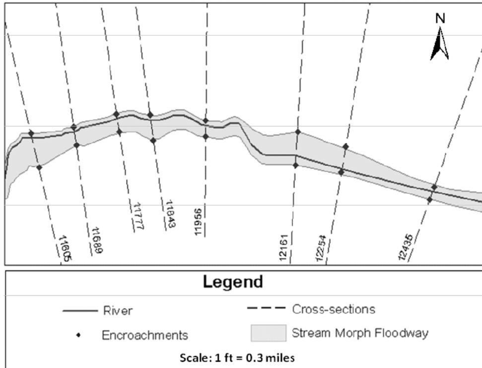
Figure 2: The stream morph mapping method. This method rubbersheets the shape of the river on either side based on the encroachment station points at each cross-section
