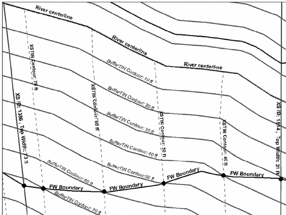
Figure 5: Overlay of the BufferTIN and XSTIN contours showing the points of intersection that forms the raw floodway boundary. The linear interpolation of floodway topwidths between cross-sections is indicated by the contours derived from XSTIN
