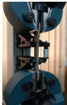
FIGURE 3. D638 LOADED IN TENSILE TESTING MACHINE
