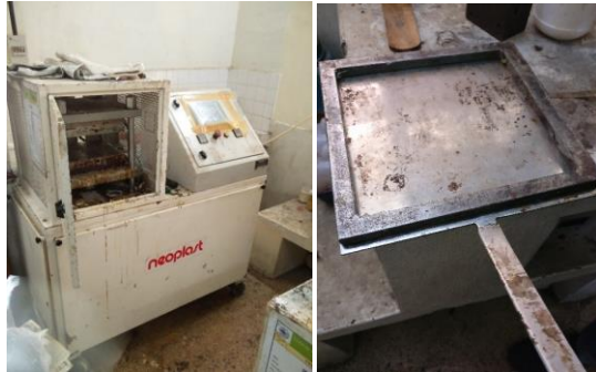
FIGURE 5 (A,B) A. COMPRESSION MOULDING MACHINE, B. MOULD
