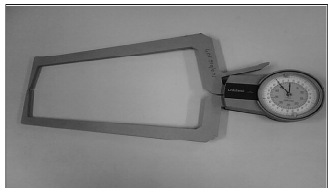
Figure 2: Inter Testing Machine for Measuring Thickness
