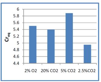
Figure 4: Chromium Equivalent (Creq) for various shielding gas
