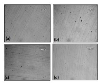
Figure 10: Weld inclusion (a) Argon + 2% O<sub>2</sub>, (b) Argon + 20% CO<sub>2</sub>, (c) Argon + 5% CO<sub>2</sub> (d) Argon + 2.5% CO<sub>2</sub>
