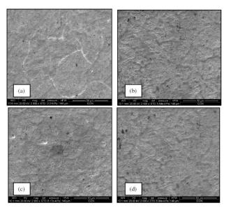
Figure 8: SEM image Before PWHT (a) Argon + 2% O<sub>2</sub>, (b) Argon + 20% CO<sub>2</sub>, (c) Argon + 5% CO<sub>2</sub> (d) Argon + 2.5% CO<sub>2</sub>
