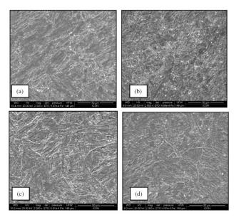
Figure 9: SEM image After PWHT (a) Argon + 2% O<sub>2</sub>, (b) Argon + 20% CO<sub>2</sub>, (c) Argon + 5% CO<sub>2</sub> (d) Argon + 2.5% CO<sub>2</sub>
