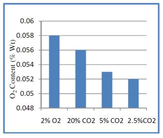
Figure 3: O2 Content for various shielding gases
