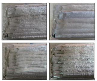
Figure 2: Bead appearance (a)Argon + 2% O<sub>2</sub>, (b) Argon + 20% CO<sub>2</sub>, (c)Argon + 5% CO<sub>2</sub>, (d) Argon + 2.5% CO<sub>2</sub>
