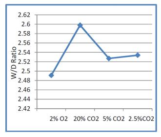
Figure 7: W/D Ratio for various shielding gas
