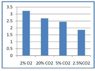
Figure 5: Ferrite factor for various shielding gas
