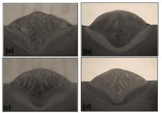
Figure 6: Bead profile (a) Argon + 2% O<sub>2</sub>, (b) Argon + 20% CO<sub>2</sub>, (c) Argon + 5% CO<sub>2</sub>, (d) Argon + 2.5% CO<sub>2</sub>
