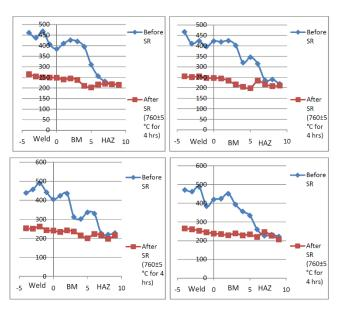
*Figure 12: Hardness survey before and after PWHT (a) Argon* + 2% *O*<sub>2</sub>*, (b) Argon* + 20% *CO*<sub>2</sub>*, (c) Argon* + 5% *CO*<sub>2</sub> *(d) Argon* + 2.5% *CO*<sub>2</sub>
