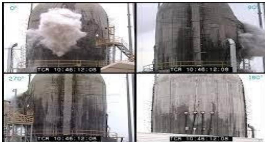
Figure: 3 The NUPEC/NRC PCCV model tested by Sandia National Laboratory
