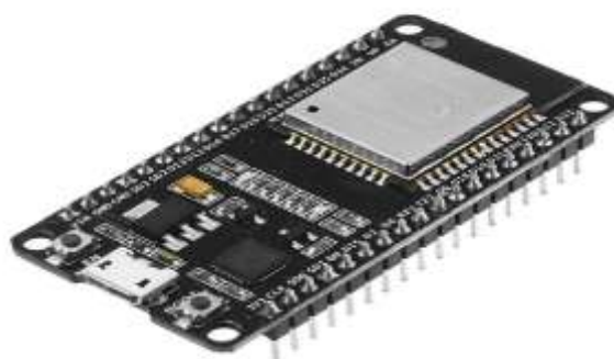
Figure: 5 The ESP32 DEVKIT V1 board used as controller
