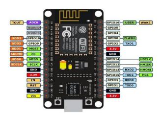
Node MCU has inbuilt WIFI which enables communication with mobile devices by connecting the node MCU with a mobile application. It is a low-cost wifi inbuilt chip used for multipurpose IoT applications.
