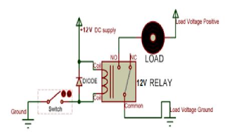
A relay is a device that opens or closes contacts to trigger the operation of another electrical controller.
