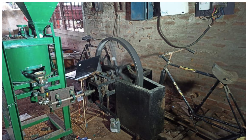
FIGURE 3. Developed experimental set-up of Miniature pulse machine energized by HPFM
