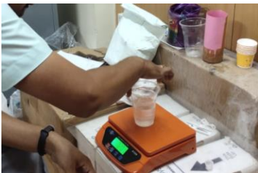
(a) Measuring of epoxy
