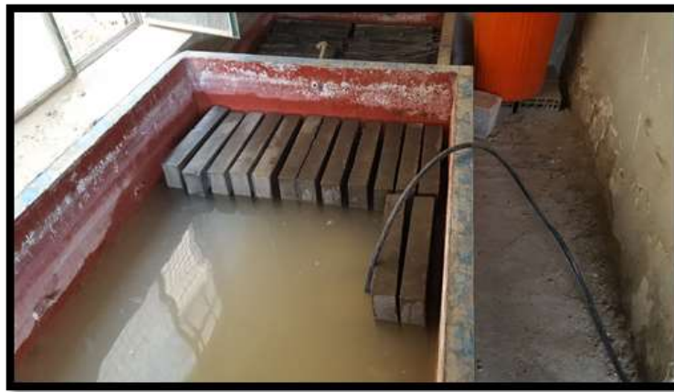
Figure 6. Slabs during curing.
