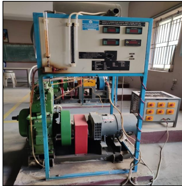
Fig. 1. Engine setup is a single-cylinder Kirloskar bore, stroke length mounted on the same base frame with eddy current.
