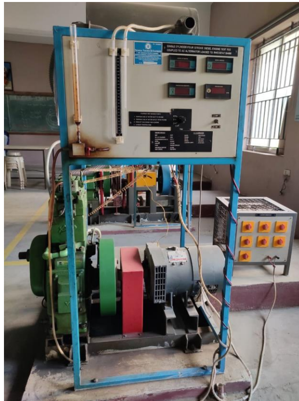
Fig. 1. Engine setup is a single-cylinder Kirloskar bore, stroke length mounted on the same base frame with eddy current.
