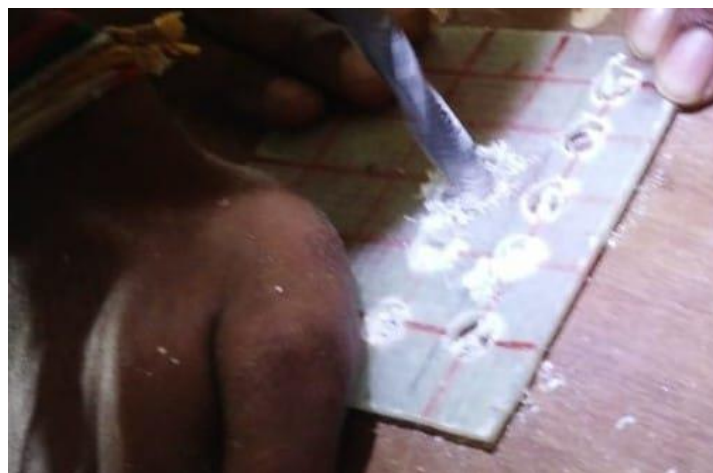
Fig. 3. Radial drilling undergone on glass fiber specimen
