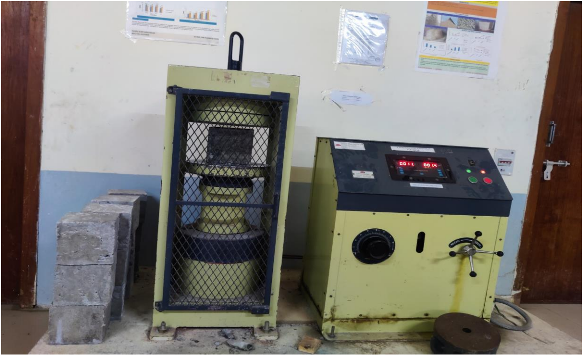
Fig.2 : Compression testing machine used to collect the compressive strength data.
