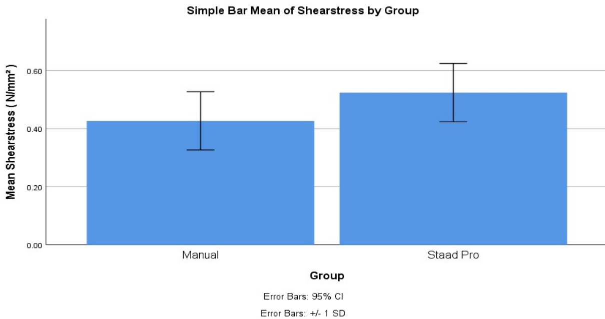
Fig. 2 Bar plot showing the mean Shear Stress(N/mm 2 ) plotted for the two groups considered, manual and STAAD Pro. The mean shear stress by STAAD pro has better accuracy than manual. X-axis: Group and Y-axis: Shear Stress(N/mm 2 ).
