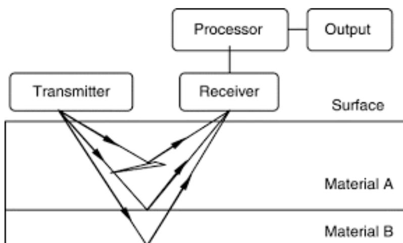
Fig. 2 Working of GPR scanner
