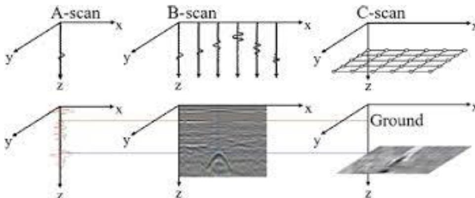
Fig.3 Different Type of Scans Used for Infrastructure Mapping
