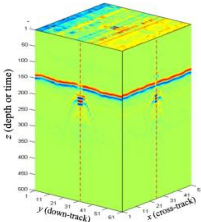
Fig 1. Three-Dimensional Rendering of data from GPR scan at a surface level
