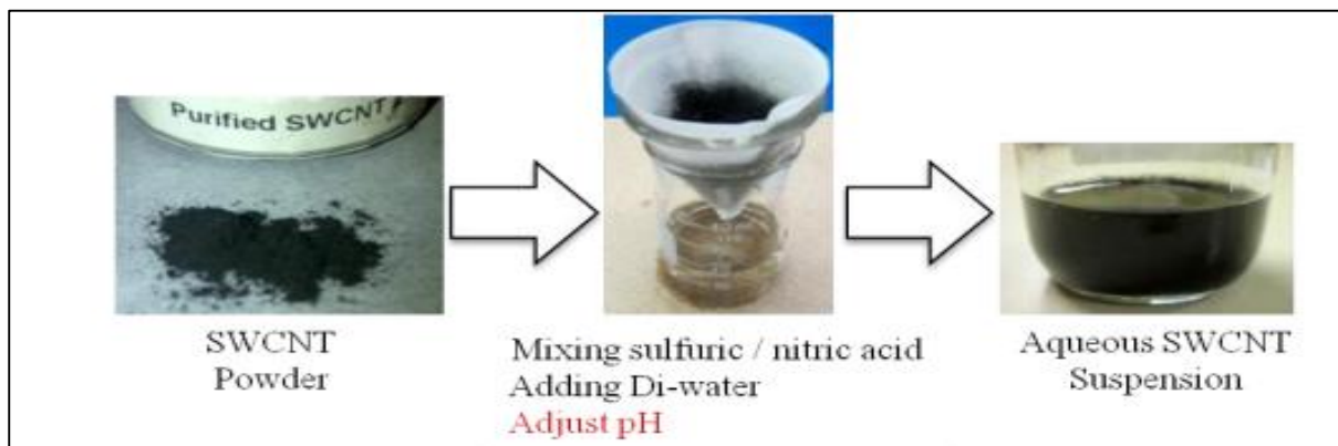
Fig. 2 Functionalization processing for SWCNTs
