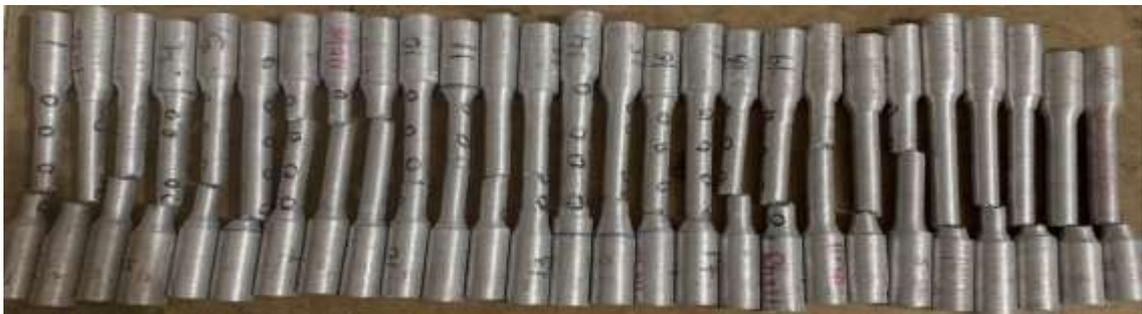
Figure 1 Tensile Tested samples
