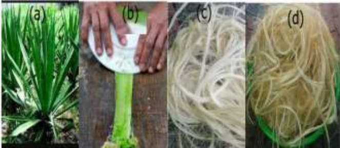
Figure 2: (a) Sisal plant (b) Extraction of Fiber (c) Untreated sisal fiber (d) kerosene treated sisal fiber
