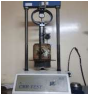
Figure 4: CBR test setup
