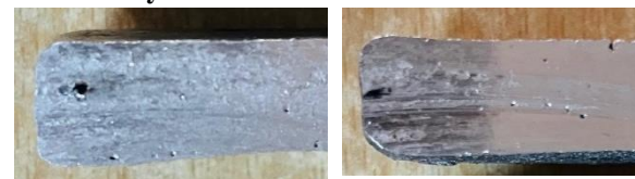
Fig. 1: Porosity in stir casted Al6061 + SiC (5 %wt) sample
