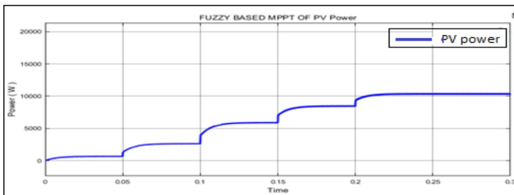
Figure 6: PV power generated using Fuzzy based MPPT
