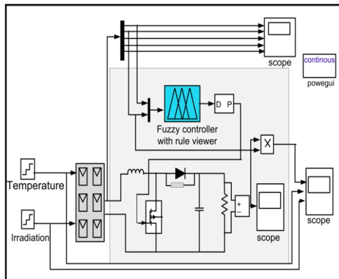
Figure 1: Simulation version for 10 kW device the use of FL MPPT controller
