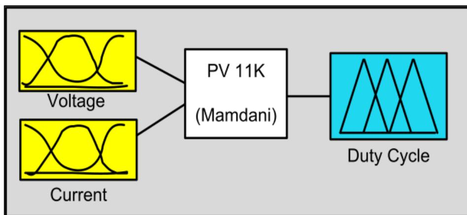
Figure 2: Fuzzy controller structure for MPPT controller
