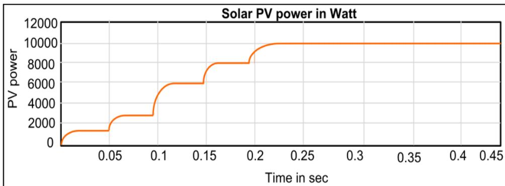
Figure 4c: PV power variation for variable irradiance and temperature
