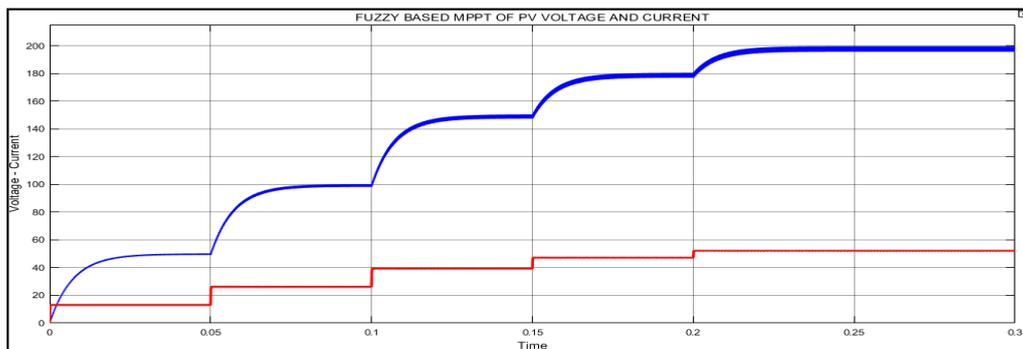
Figure 5: PV voltage and current of Fuzzy based MPPT
