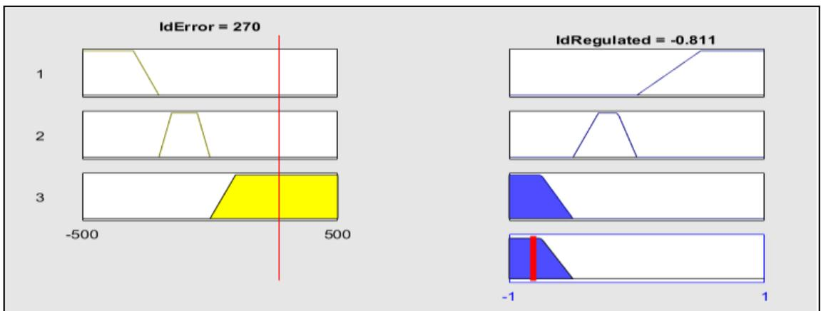
Figure 13: Fuzzy membership functions for DFIG controller
