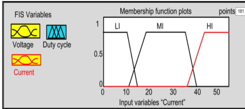
Figure 3b: Input Fuzzy membership functions for PV MPPT FL
