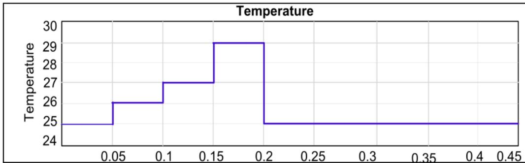
Figure 4b: PV temperature variation with time
