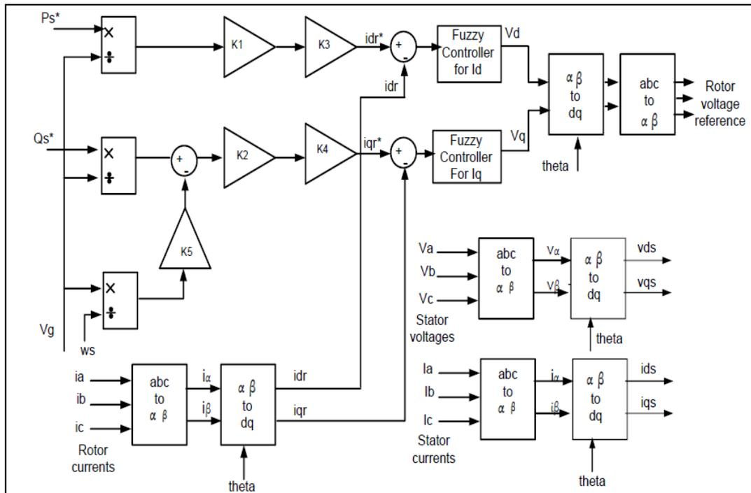
Figure 10: Calculation of the current references required for rotor converter
