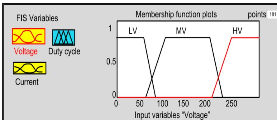
Figure 3a: Input Fuzzy membership functions for PV MPPT FL
