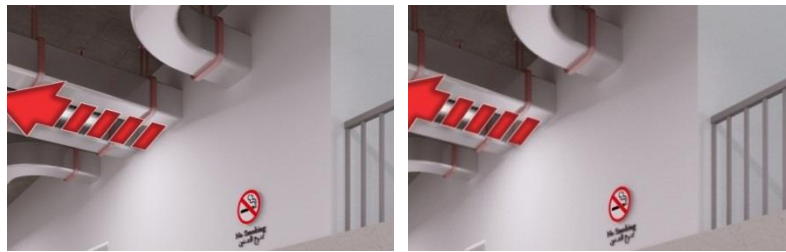
Fig. (39): Air ducts exiting the service skylight and distributing them to the right and left of the classrooms and administrative spaces.
