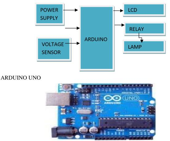
The **Arduino Uno R3** is a microcontroller board based on the ATmega328 (<u>datasheet</u>). It has 14 digital input/output pins (of which 6 can be used as PWM outputs), 6 analog inputs, a 16 MHz crystal oscillator, a USB connection, a power jack, an ICSP header, and a reset button. It contains everything needed to support the microcontroller; simply connect it to a computer with a USB cable or power it with a AC-to-DC adapter or battery to get started.
