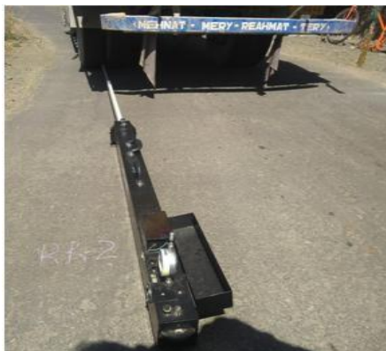
Fig 2 Benkelman Beam Deflection study on selected stretches (NRR-2)
