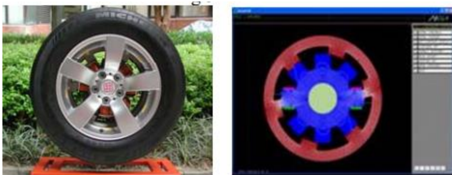
Figure 3. The in-wheel motor a) Hardware b) FEM model
