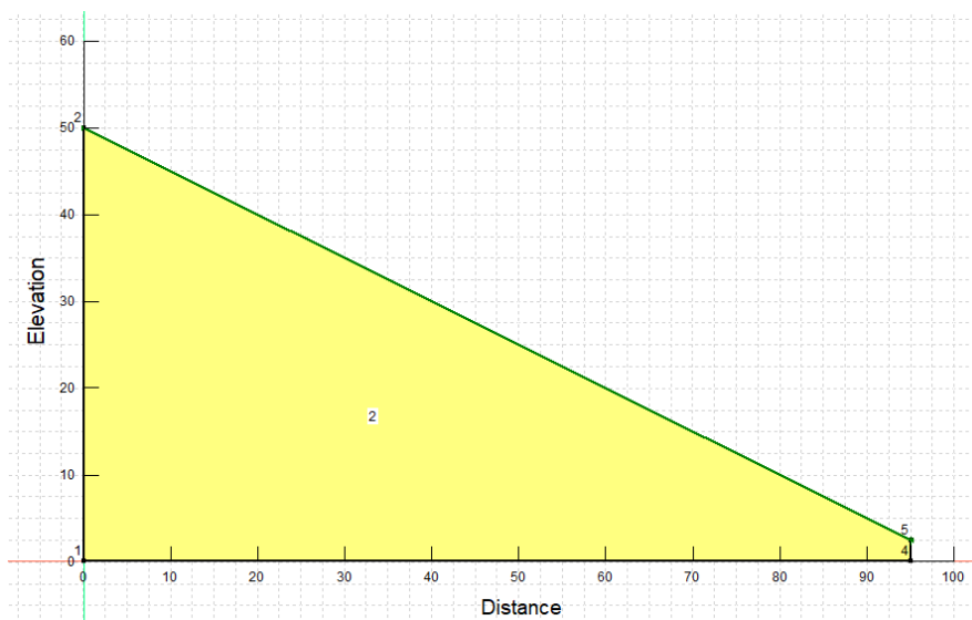
Fig-1 Geometry of the slope model for 25° slope angle with 5 m toe excavation
