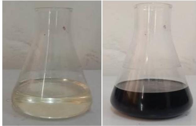
Figure 3 picture of pure POE oil and synthesized MWCNT nano oil at a mass fraction of 0.3%
