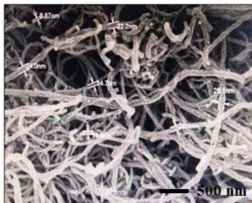
Figure 2 Scanning electron microscopy (SEM) of MWCNT nanoparticles
