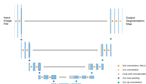
Figure 1: Basic U-net architecture
