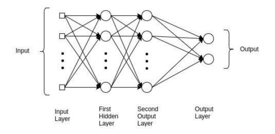
According to the learned features the classification operations have been done. The number of hidden layers has been chosen by the designers of the model according to the complexity of the problem addressed. The hidden layers consist of neurons. The neurons have been trained using the back propagation learning algorithms. The Multi-Layer Perceptron (MLP) model is very useful for this task.
