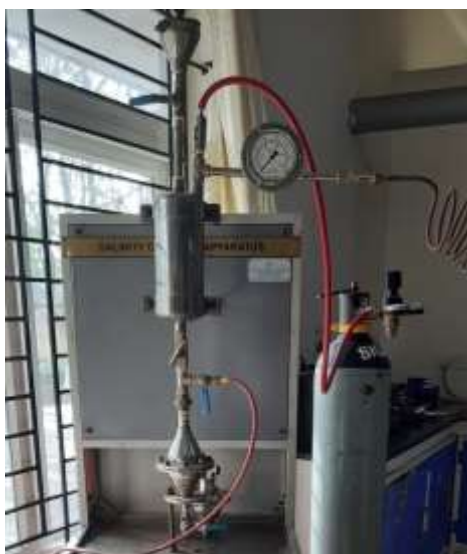
Fig. 6. Digital photograph of lab made flux- rejection equipment
