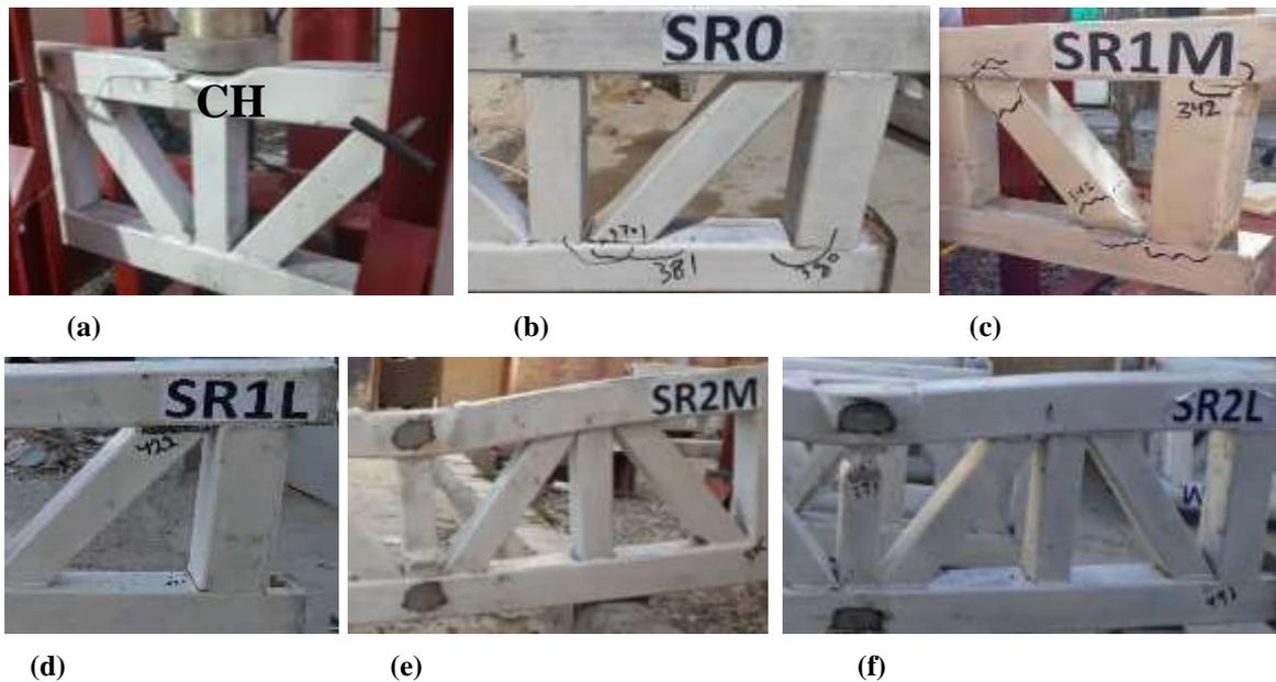
**Figure-10** Modes of failure.
