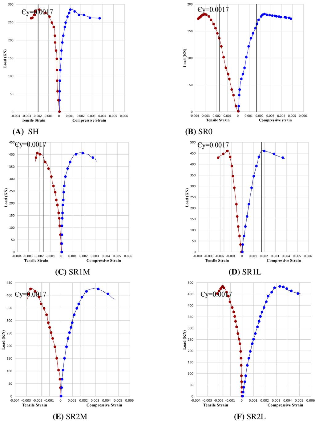
**Figure -8** distributions of the longitudinal strain for the chords at the midspan for all specimens.
