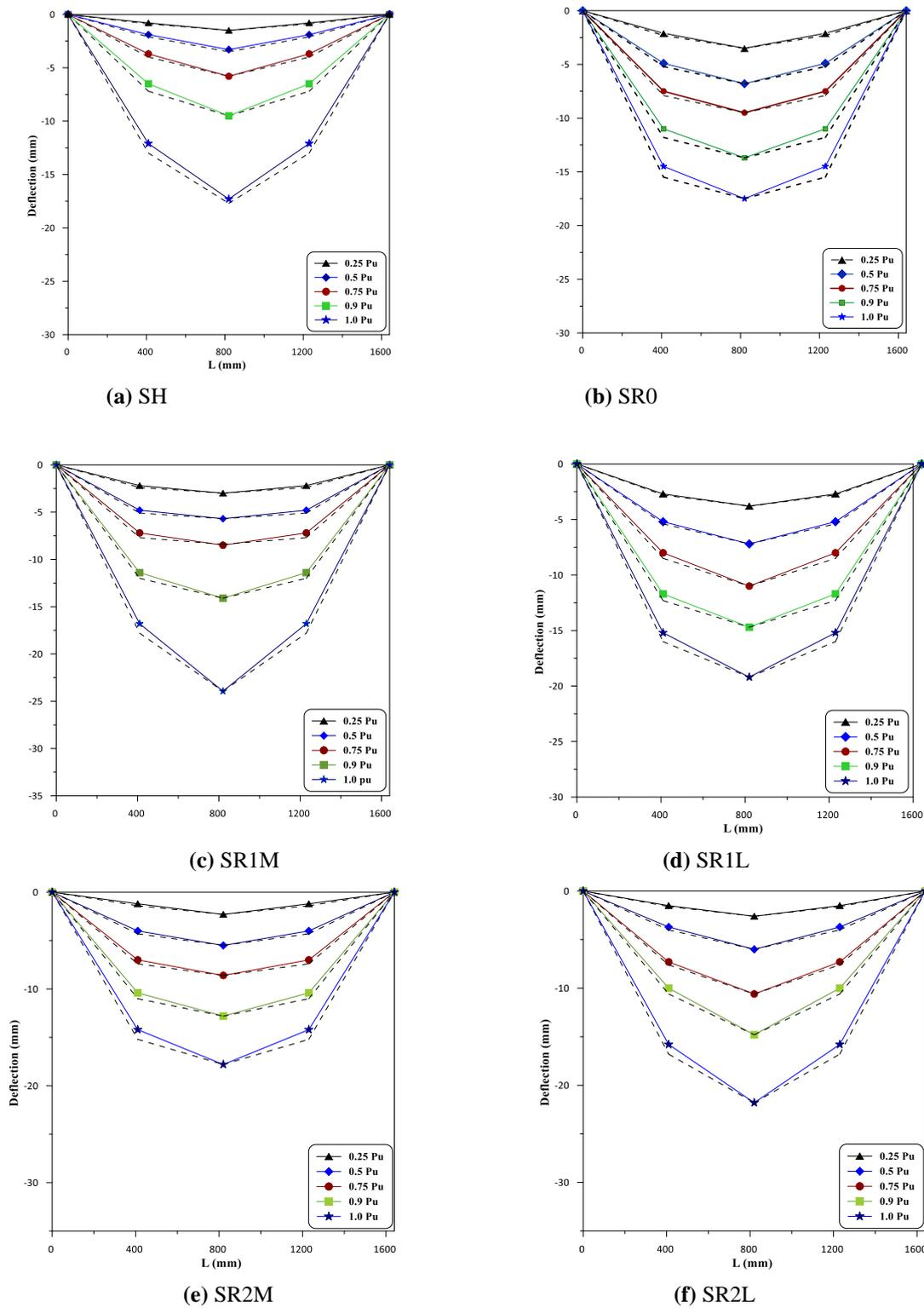
**Figure -9** Deflections along span about different loading levels.
