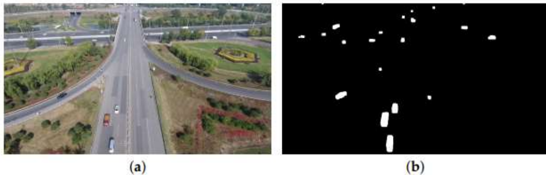
Figure 7. Post-processing examples (static background). Images are post-processed using the median filter. This segmented image had noise in it, so we chose an area to filter to reduce that noise: (a) the original image; and (b) the final result of detector.
