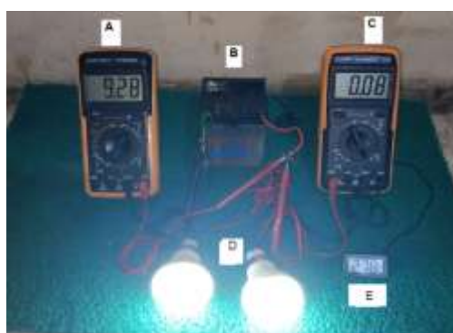
Figure 4. Bio Moringa Cell Accumulator Electrolyte Testing on LED lamps
