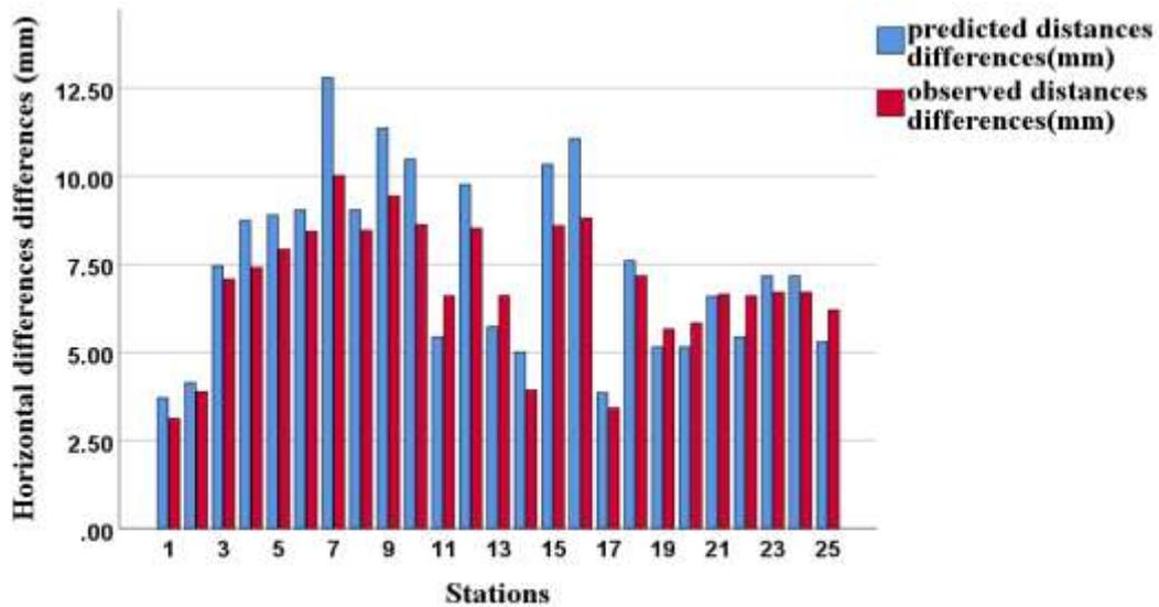
**Figure (4.5): The observed and predicted horizontal distances differences histogram for each measured station with the upstream side of the dam during (2016-2017)**
