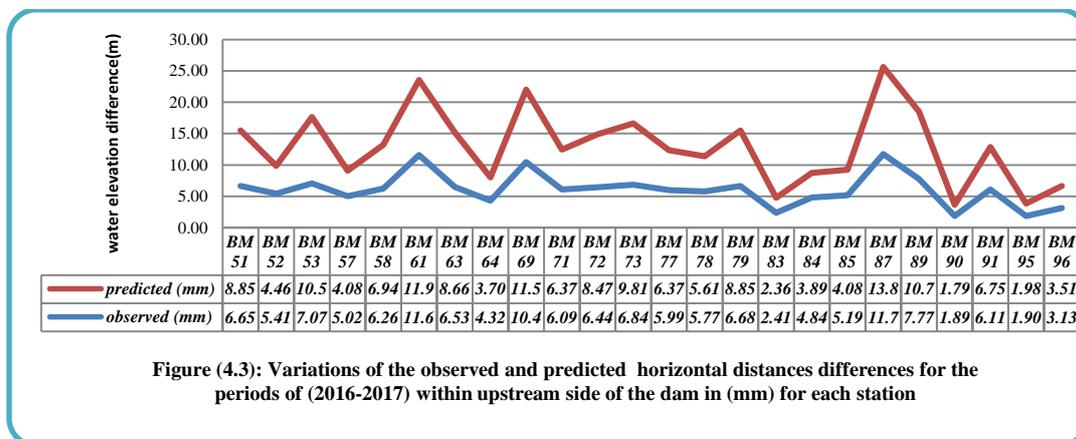
Figure (4.3): Variations of the observed and predicted horizontal distances differences for the periods of (2016-2017) within upstream side of the dam in (mm) for each station
