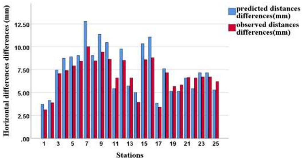
**Figure (4.6): The observed and predicted horizontal distances differences histogram for each measured station with the downstream side of the dam during (2016-2017)**
