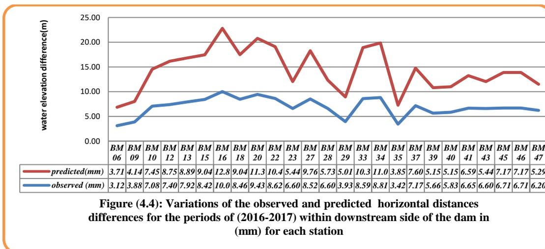
Figure (4.4): Variations of the observed and predicted horizontal distances differences for the periods of (2016-2017) within downstream side of the dam in (mm) for each station
