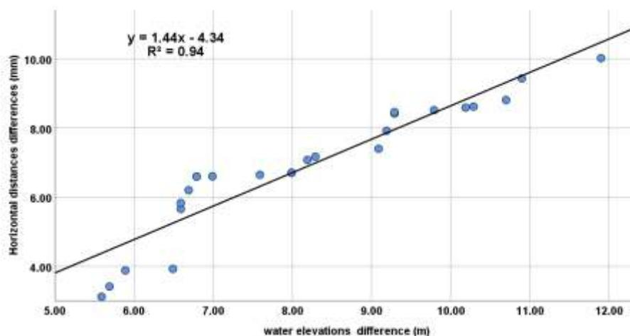
Figure (4.2): Relation model of horizontal distances differences (creep) versus (water elevations head difference) for the period of (2016-2017) within downstream side of the dam
