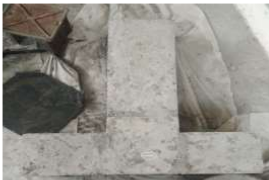
Fig 6. Sample specimen for bamboo beam - column Joint
