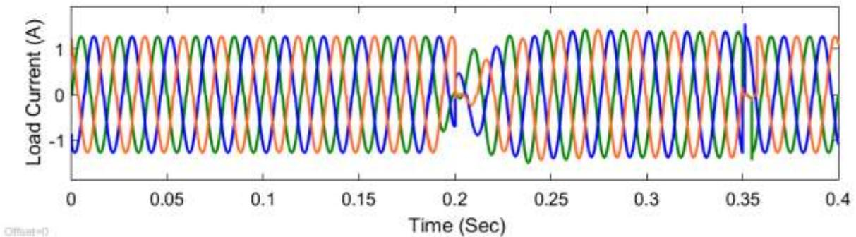
Fig.12: With ZDVR Output Load Current (A)
