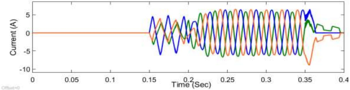
Fig.7: Compensating Current wave form RL LOAD LLLG Fault
