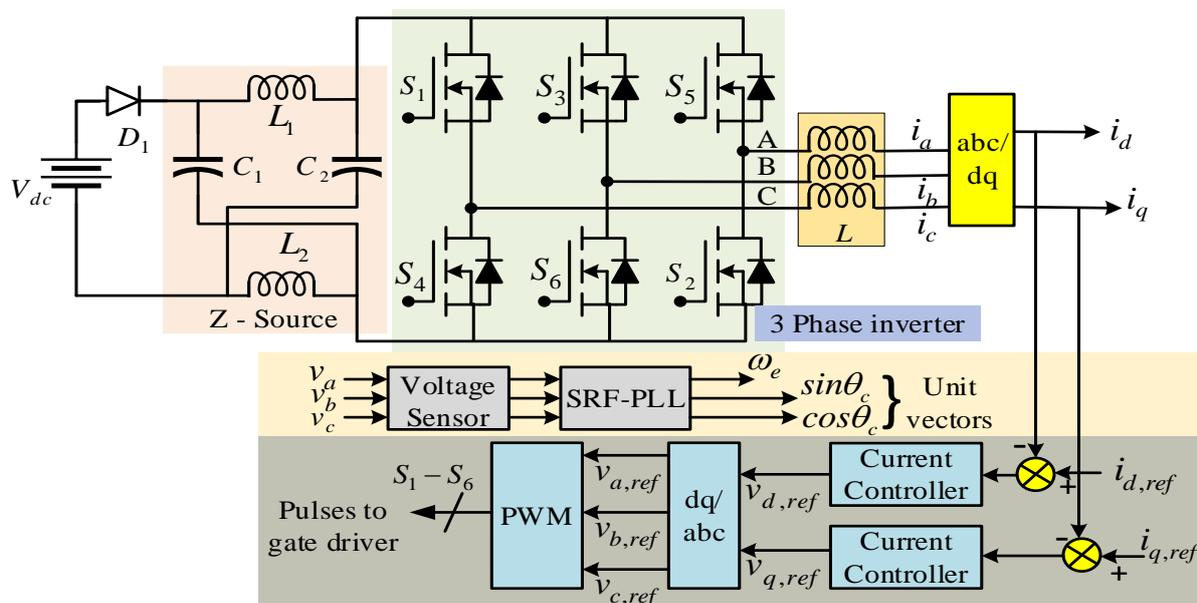
Fig.3: SRF controller based Z-DVR
