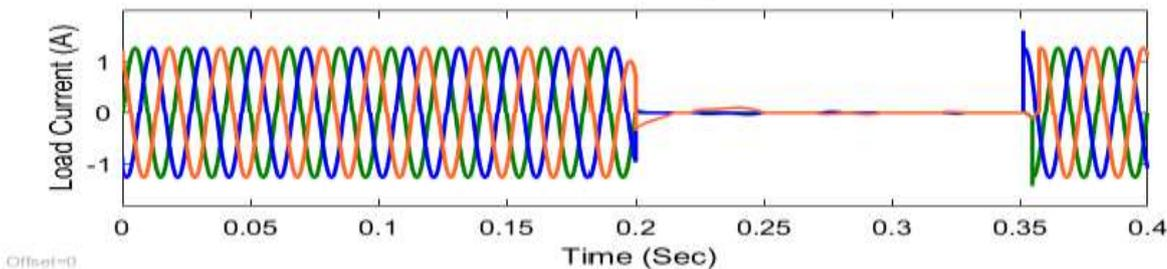
Fig.5: Sag on feeder Without Z DVR RL Load LLLG Fault
