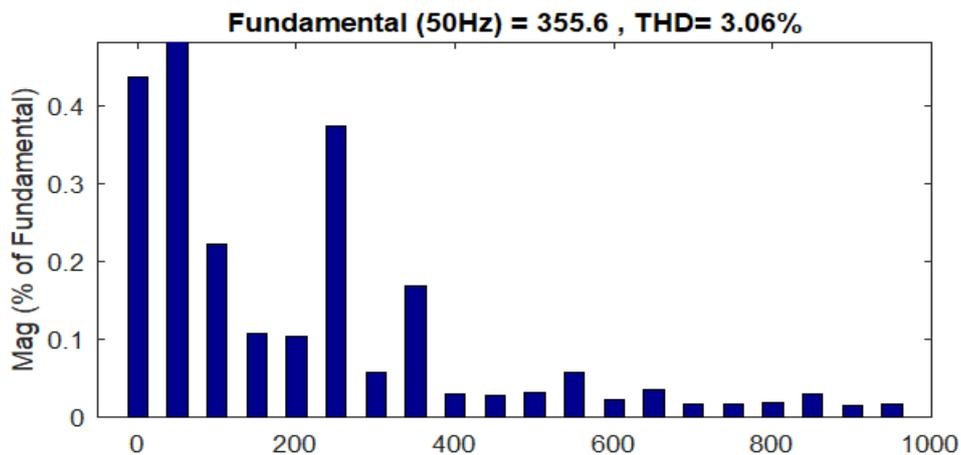
Fig. 13: THD of load voltage after compensation
