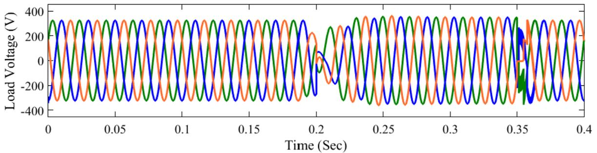
Fig.11: With ZDVR Output Load Voltage (V)
