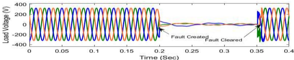
Fig.4: Voltage sag on feeder Without Z DVR RL LOAD LLLG Fault
