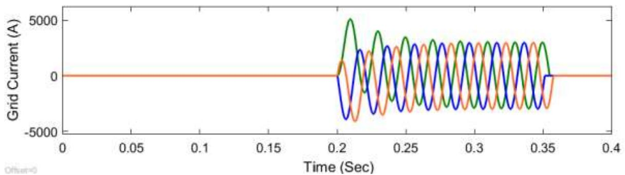
Fig.10: Current sag on feeder Without Z DVR RL LOAD LLLG Fault
