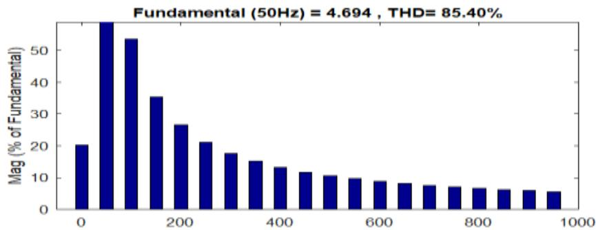
Fig.8: Without ZDVR THD VALUE RL LOAD LLLG Fault
