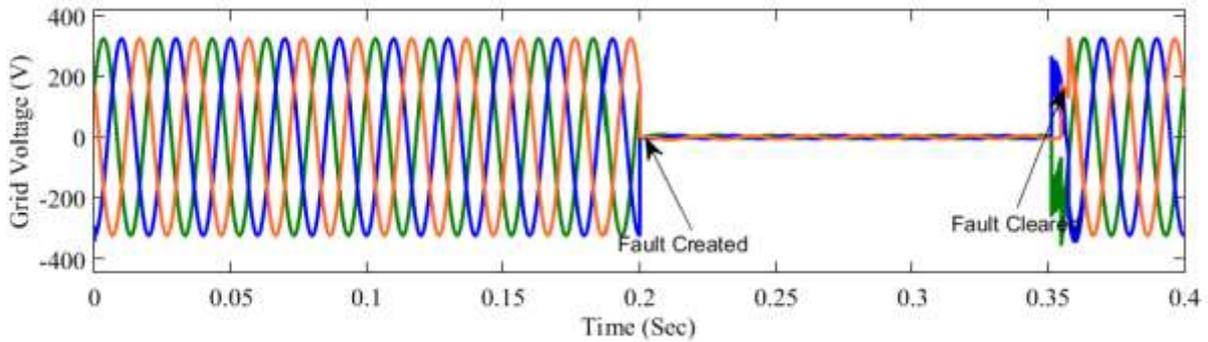
Fig.9: Voltage sag on feeder With Z DVR RL LOAD LLLG Fault
