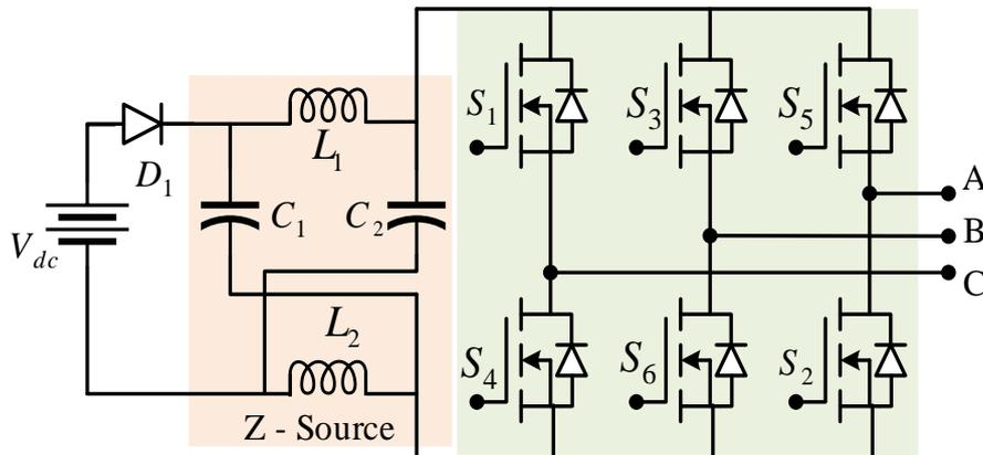
Fig. 2: Z-Source inverter in the DVR System
