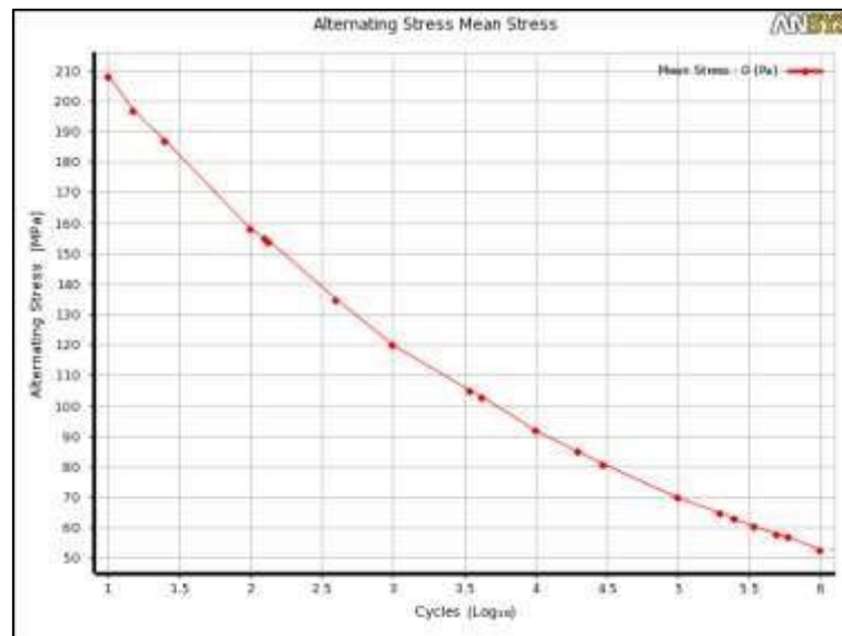
Figure 2: S-N curve for carbon fiber with lamination resin.
