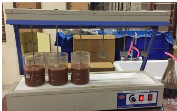
Figure 5. Beakers containing mixture with vertical axis rotary machine
