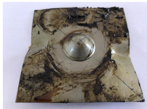
FIGURE 15. FRACTURE IN 0.5 mm THICKNESS SHEET- WET CONDITION
