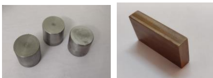
Fig 1: Workpiece and copper electrode before machining
