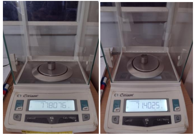
Fig 2: Weighing of samples before and after machining
