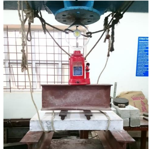
Figure 8: Wall panel being tested for flexural strength
