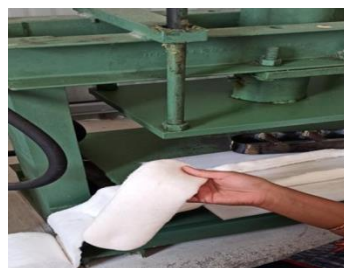
Figure 3b Mould cut sanitary napkin webs
