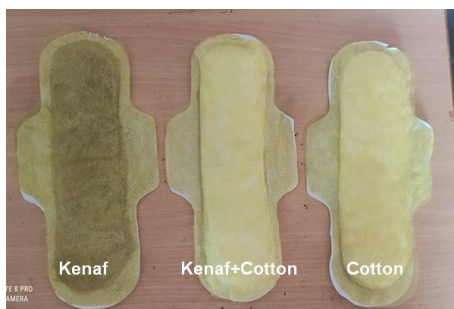
Figure 4 Prepared sanitary napkins using cotton and kenaf fibres
