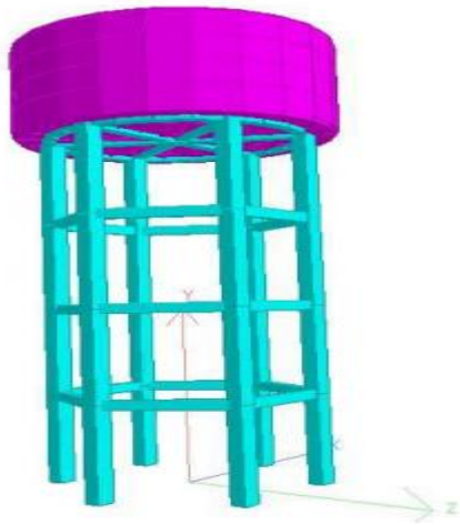
Figure1: 3D model of Elevated Circular Tank
