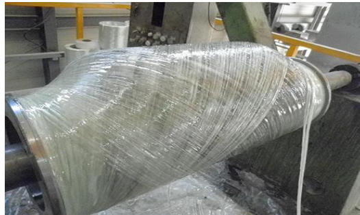
Figure 7. Fiberglass adhesive mixed winding scene
