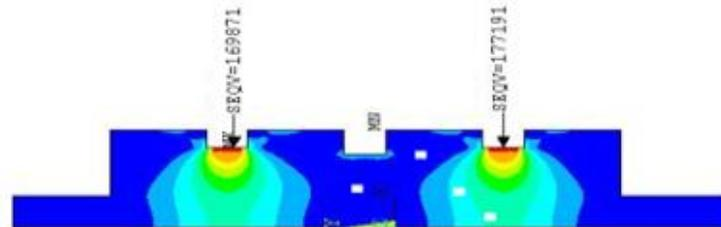
Fig. 11 Bending stress of HPT rotor
