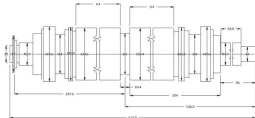
Fig. 3 Line diagram of LPT rotor
