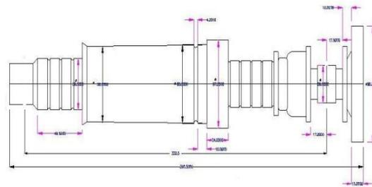
Fig. 1 Line diagram of HPT rotor
