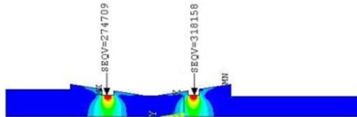
Fig. 10 Bending stress of HPT rotor
