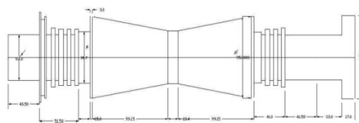
Fig. 2 Line diagram of IPT rotor
