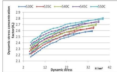
Fig. 13 Dynamic stress concentration factor based on dynamic stress
