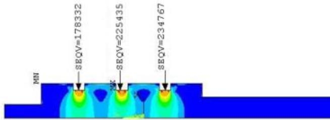
Fig. 9 Bending stress of HPT rotor
