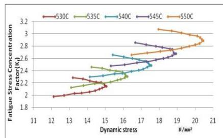
Fig. 14 Dynamic stress concentration factor based on dynamic stress
