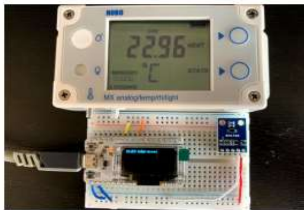
Fig. 2 The light intensity data logger of the MX1101 is connected to the ESP32 development panel and the ambient light sensor BH1750.
