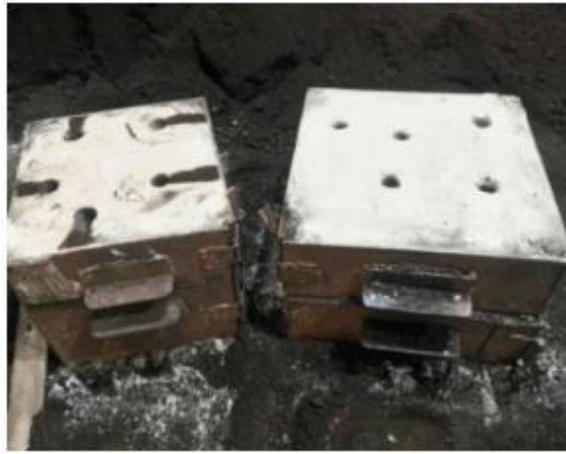
Fig. 2: MOULD CAVITY FOR CASTING PROCESS
