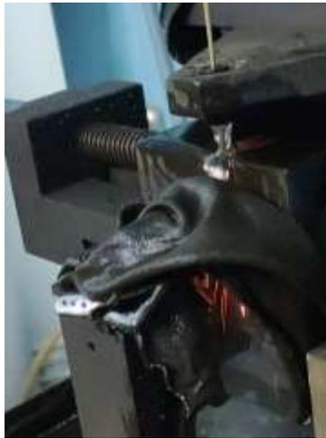
Fig. 14. EDM process
