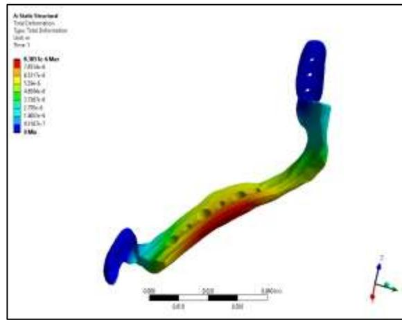
Fig. 8. Deformation of the redesigned model
