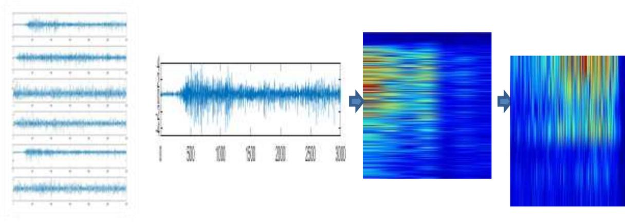
Figure5. The process of transforming EMG signals to EMG images BY CWT.
