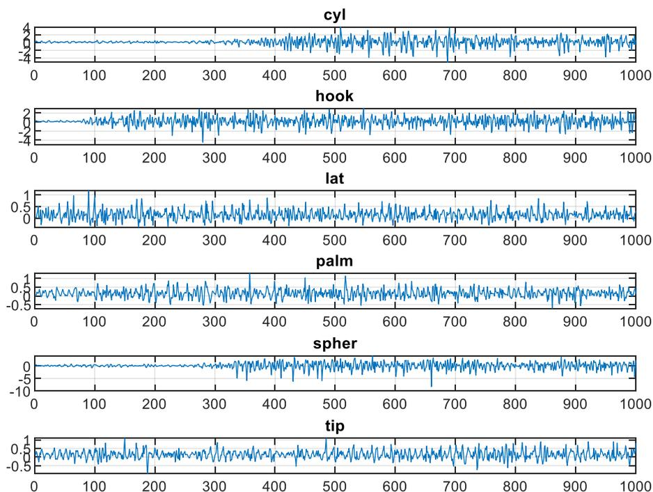
fig. 2. Typical forms of EMG signals matching to hand grips. A EMG signals is: cyl, hook , lat ,palm, sphere and tip
