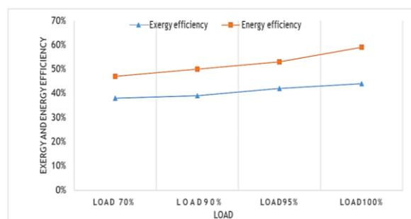
Fig. 2. Energy and exergy efficiencies vs. generator output (load)
